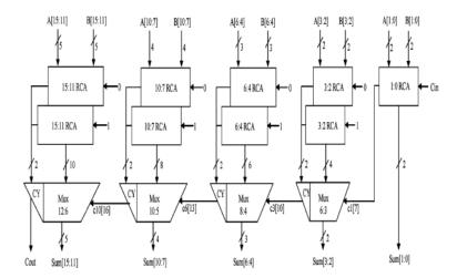
Through searching the truth table of a single bit full adder, to find out the output of summation signal as carry-in signal is logic '0' is the converse signal of itself as carry-in signal is logic '1'. By sharing the common Boolean logic term in addition generation, a proposed carry select adder design is illustrated in figure.
