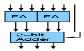
Wallace multiplier is an efficient parallel multiplier. In the current Wallace tree multiplier, the first step is to form unfinished product array (of N2 bits). In the second step, groups of three nearest rows each, is collected. An adder tree to add three 4-bit numbers is shown below:
