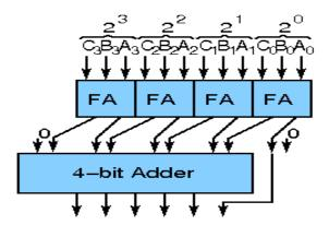
Each group of three rows is redacted by using full adders and half adders. Full adders are used in each column where there are three bits whereas half adders are applicationwise in each column where there are two bits. Any single bit in a column is passed to the next level in the same column without processing. This reduction procedure is repeated in each successive stage until only two rows balance. In the final step, the balance two rows are added using a carry propagating adder.
